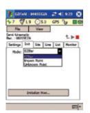
The key requirement for achieving centimeter accuracy with a GNSS-L1 receiver is to initialize your survey prior to moving the antenna. Initializing a survey means determining the carrier phase ambiguities.
